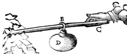
The use of the lever explained above placed the weight at one of its extremities and the force at the other, while the support was placed somewhere between the extremities. But we can use the lever in another way too, placing the support at the extremity A (as seen in the diagram), the force at the other extremity C, and hanging the weight D from some point between, as at the point B.
