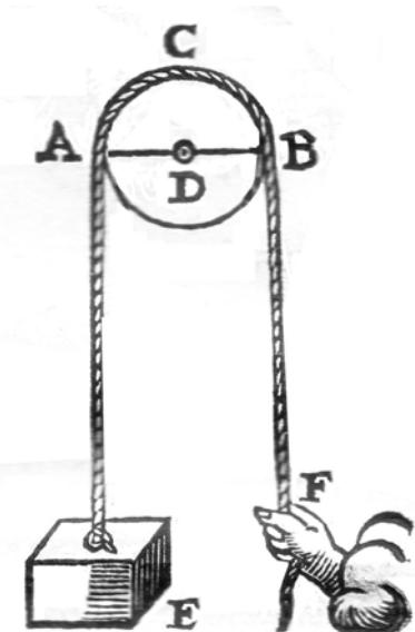
And first think of the pulley ABC made of metal or hard wood, turning about its axle that passes through the center D; and round this pulley place the cord EABCF, from one end of which hangs the weight E, and at the other assume the force F. I say that the weight will be sustained by a force equal to itself, nor will the upper pulley ABC give any benefit with regard to moving or sustaining the said weight with the force placed at F ...considered simply, but only in the mode of applying it.
