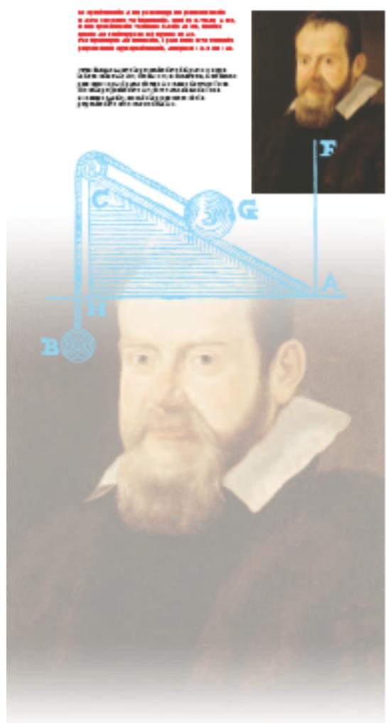
From the point C, let fall the perpendicular CH upon the horizontal line AR. It will be demonstrated that the same weight will be moved upon the inclined plane AC by less force than in the perpendicular AF (where it will be raised by a force equal to itself), in proportion as the perpendicular CH is less than AC.
