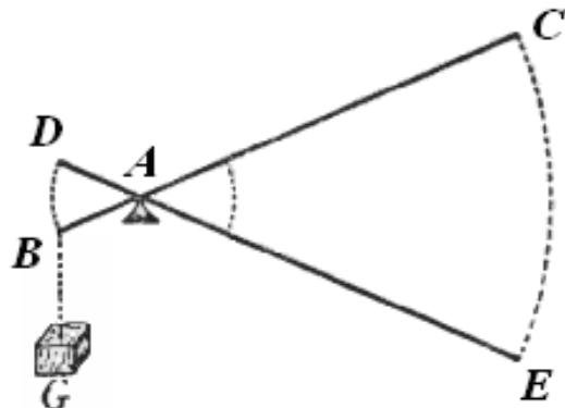
The two instruments whose nature we are now about to explain depend directly upon the lever, and indeed are nothing but a perpetual lever. For if we think of the lever BAC supported at the point A, and the weight G hanging from the point B, the force being placed at C, it is evident that by transferring the lever to the position DAE, the weight G will rise through the distance BD, but that it cannot continue to be elevated much more.
